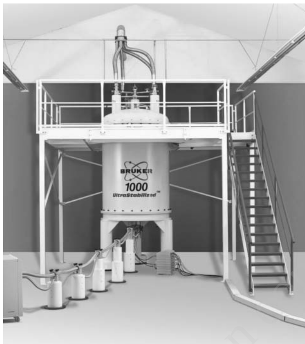
Figure 15.35 Laboratory with a superconducting magnet of 1 GHz ^1\text{H} NMR frequency. The superconducting coil is held at approximately 2 K by use of an additional Joule-Thompson valve (Courtesy: Bruker BioSpin, Karlsruhe, Germany).
